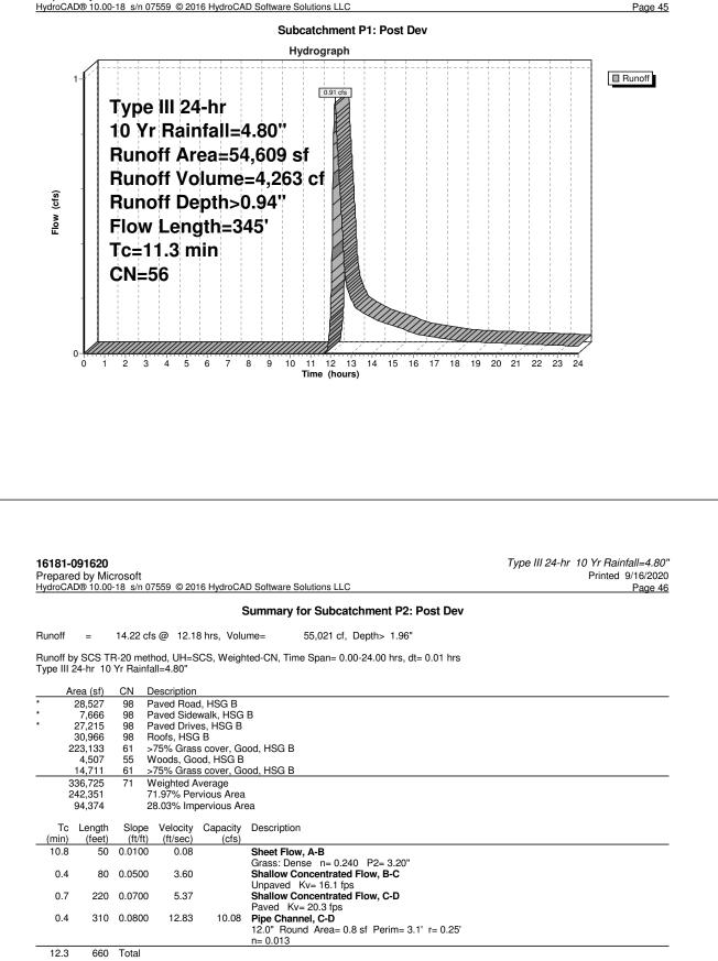
16181-091620 Prepared by Microsoft HydroCAD® 10.00-18 s/n 07559 © 2016 HydroCAD Software S
