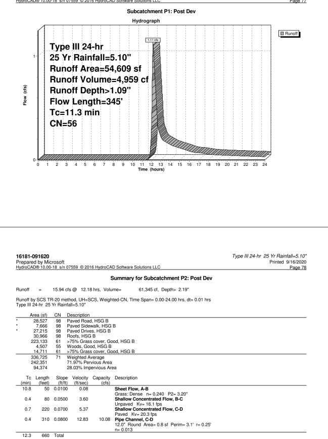
16181-091620 Prepared by Microsoft HydroCAD® 10.00-18 s/n 07559 © 2016 HydroCAD Software Solutions LLC
