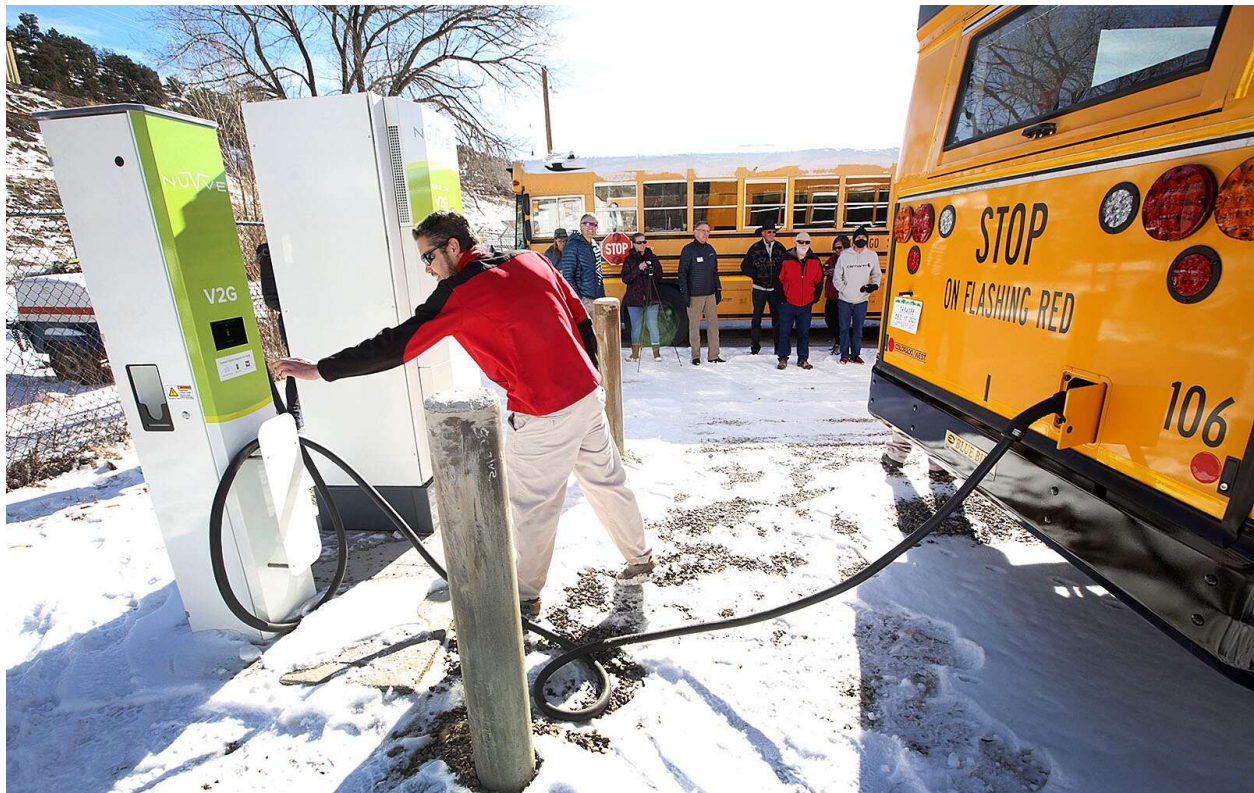
Figure 20. Durango, Colorado school bus V2G installation 29
