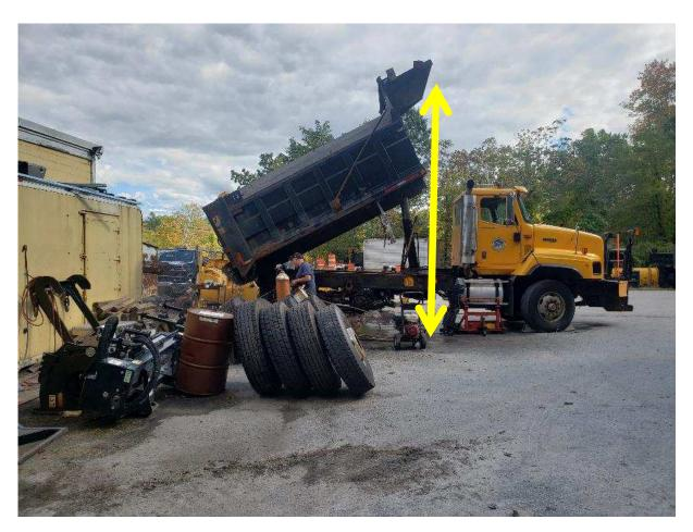
Inadequate height to raise a dump body inside for maintenance
