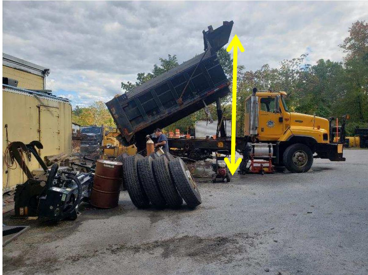
*Inadequate height to raise a dump body inside for maintenance*
