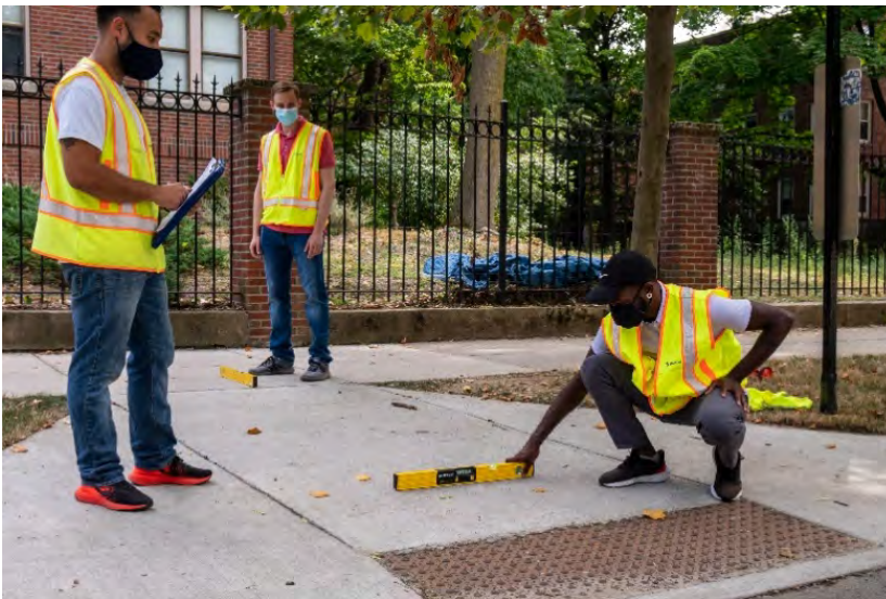
Recording ramp slope(s) in field
