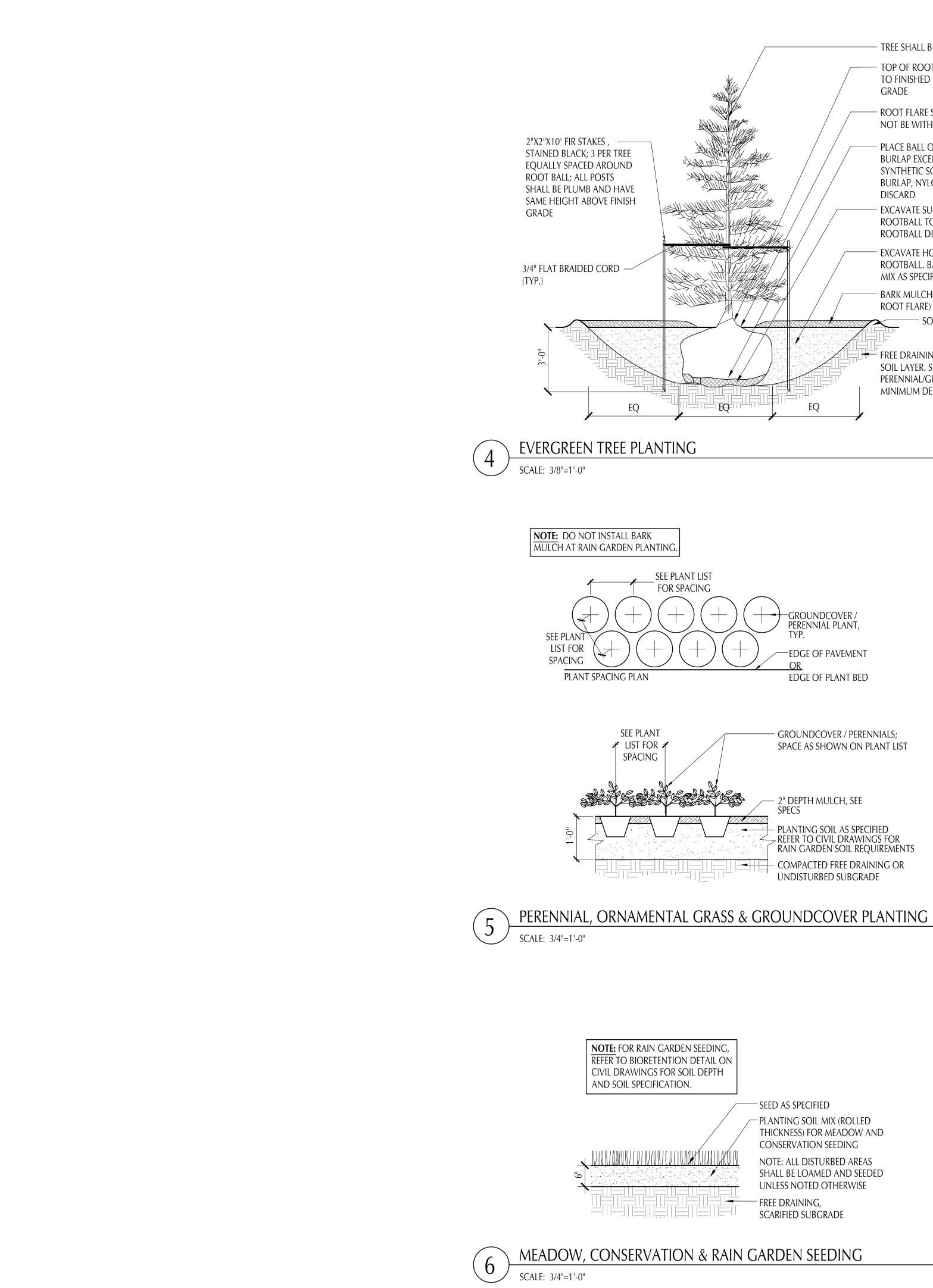
3/4" FLAT BRAIDED CORD (TYP.) -2:1 MAX SLOPE **GROUNDCOVER / PERENNIALS;** SPACE AS SHOWN ON PLANT LIST - PLANTING SOIL AS SPECIFIED - REFER TO CIVIL DRAWINGS FOR RAIN GARDEN SOIL REQUIREMENTS COMPACTED FREE DRAINING OR UNDISTURBED SUBGRADE SCALE: 3/8"=1'-0" THICKNESS) FOR MEADOW AND SHALL BE LOAMED AND SEEDED
