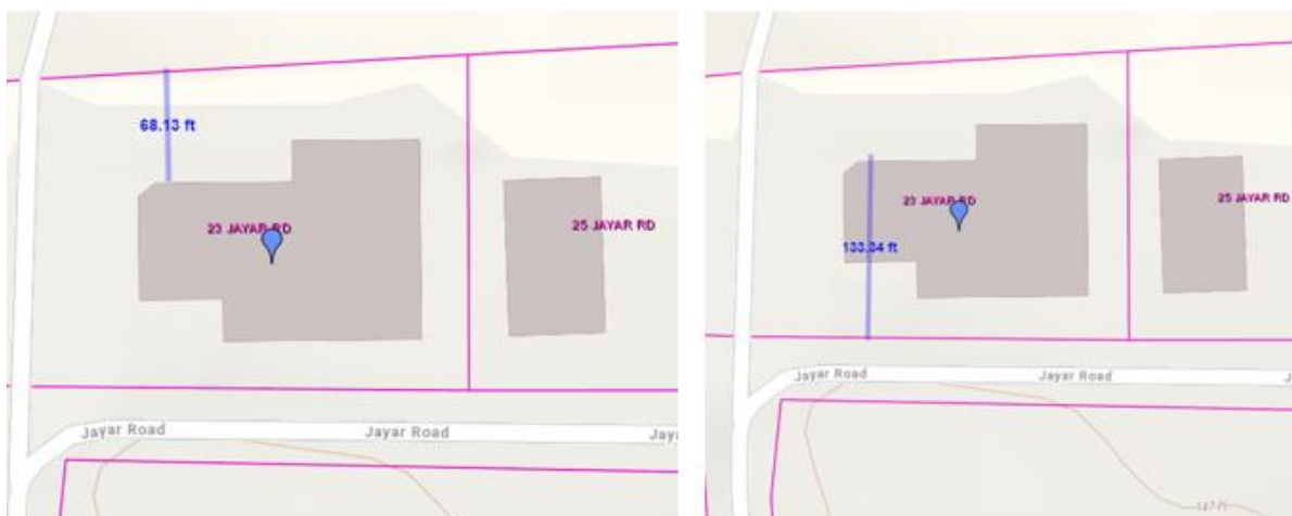
Figure 2. Distance of proposed chiller and generator units to closest property lines
