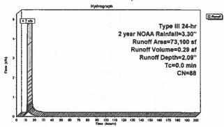
Type III 24-hr 2 year NOAA Rainfall=3.30\* **Lowland Street 2022** Prepared by Microsoft HydroCAD® 10.10-7a sh 01413 © 2021 HydroCAD Software Solutione LLC Printed 10/21/2022
